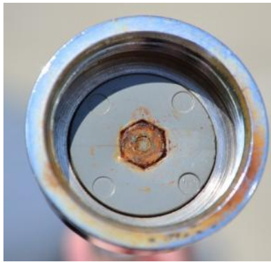
Unscrew antenna from vehicle & inspect the underside - a rusty base prohibits transmission & reception!
