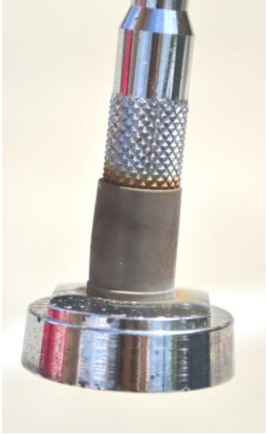
Plastic DUELIST can dry out and split, metal will rust on your mobile antenna
